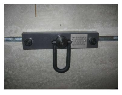
THE STRUT RIGGING PICK POINT HAS A WLL OF 2,000 LBS VERTICAL AND 1,000 LBS IN ANY DIRECTION AND CAN BE INSTALLED ON ANY STRUCTURE THAT HAS PRE-INSTALLED UNISTRUT OR SIMILAR STRUT TRACK. THIS RIGGING PICK POINT ATTACHES DIRECTLY TO THE STRUT TRACK.
